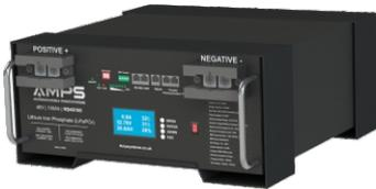
This is a 48V (51.2V) 100Ah lithium iron phosphate battery. This stores 5.12kWh of capacity. Put simply, this delivers 5kW of power for 1 hour. These can be stacked in parallel to increase capacity and delivery performance. 2x would be 10kW of power over 1 hour or 5kW over 2 hours. Add additional for more power and capacity.
