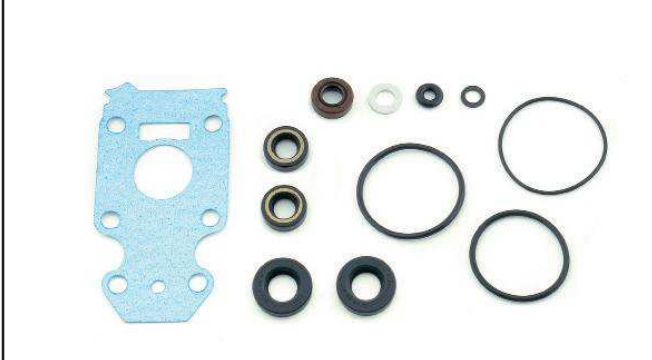
18-74544 GEAR HOUSING SEAL KIT Replaces: 68T-W0001-20-00 Fits: Yamaha F6/F8(2001-03)
