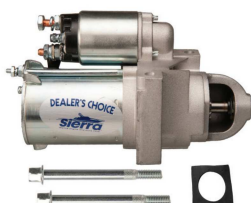
18-5913 STARTER Replaces: 3856004, 3860764, 3587625, 3853982, 3854751, 3885317 (Clockwise) Delco permanent magnet gear reduction 2 bolt starter. 12V - 11 Tooth Offset Bolt Pattern For: Late model GM 14" Flywheel SAEJ1171 1.7 KW
