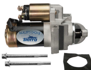
18-5913 STARTER Replaces: 3856004, 3860764, 3587625, 3853982, 3854751, 3885317 (Clockwise) Delco permanent magnet gear reduction 2 bolt starter. 12V - 11 Tooth Offset Bolt Pattern For: Late model GM 14" Flywheel SAEJ1171 1.7 KW
