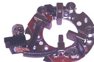
18-56009 BRUSH HOLDER ASSEMBLY Replaces: 31173-99E00 Fits: 115-140 HP 2 Stroke Use with 18-6416 Starter
