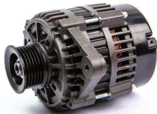
18-5984 ALTERNATOR Replaces: RA097007B 75I/70 amp, spool mount, 2 5/8" OD, 6 groove serpentine pulley Clockwise position, 65mm
