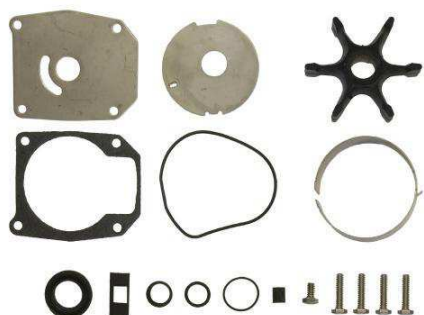
18-3387 WATER PUMP KIT Without Housing Replaces: 432956
