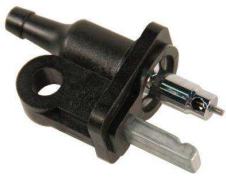
18-80407 FUEL CONNECTOR Replaces: 17710-ZW9-033 5/16" with interlocking post Fits: BF8-BF130 (2003) Mates with 18-80403, 18-80408
