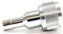
18-80401 FUEL CONNECTOR Female hose connector, new style, 3/8" hose. Will not interchange with OE's 5/16" hose assemblies. Mates with 18-80400, tank outlet
