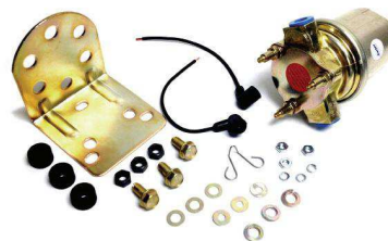
18-7333 ELECTRIC FUEL PUMP UNIVERSAL 12V, 72GPH at 5.75 PSI, 1/4" NPSF for 3/8" hose, for use with gasoline and diesel fuel. OP72533 pressure safety switch recommended.
