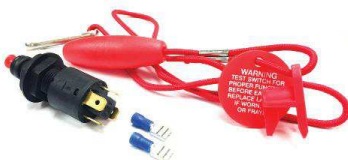
MP40960** EMERGENCY CUT-OFF SWITCH 4 terminals allow selection of normally open or normally closed circuit. Use MP40980 replacement lanyard. MP40962 "Bulk" - 100 pieces per carton
