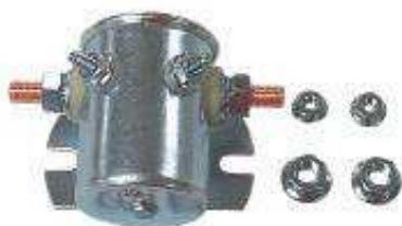
BA58003 • Use as battery isolation switch • Steel housing copper contacts • 12 Volts insulated • Continuous rating: 80 amp @ 12 VDC • Intermittent rating: 750 amp make 100 amp break 10 seconds ON 30 minutes OFF
