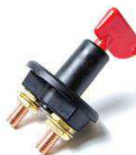
UN77310** BATTERY SWITCH Polyester housing is rust and corrosion proof. Removable plastic key for security. Two position switch "Off-On". Two 10MM X 1.5MM stud terminals. For panels up to 1.25 thick. Four mounting holes in a rectangle 1.3" and .8" on centers. 350 amp continuous rating. 500 amp intermittent rating.
