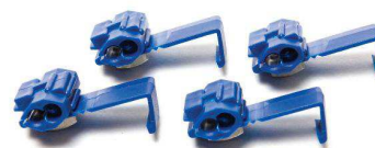
TC43904 Non-Strip Splicers Four blue non-strip splice connectors for making secure, permanent splices without stripping wires manually. Crimp with pliers and metal insert makes connection. Plastic top folds over to insulate connection.
