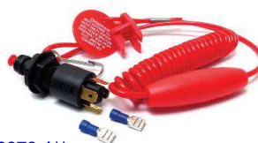
MP40970-1** EMERGENCY CUT-OFF SWITCH 4 terminals allow selection of normally open or normally closed circuit. Use MP40990 replacement lanyard. MP40972-1 "Bulk" - 100 pieces per carton.
