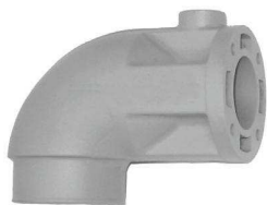
18-1928 ELBOW W/ 4" OUTLET Replaces: Crusader 97924 Crusader GM Small Block V8 305-350cu.in. (Models: 220 and 270), GM Big Block V8 454cu.in.(Models: CH350 and 454XL) 4" Hose Use with: Manifold: 18-1925, 18-1926, 18-1933, 18-1929 Elbow Gasket: 18-0309-1 Mounting Kit: 18-8515
