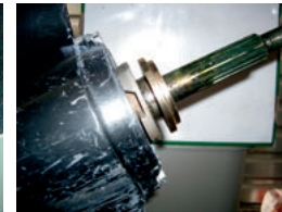
Fig. 6 OEM forward thrust washer was not removed. XHS Hub Kit and Michigan Wheel propeller will not fit properly.
