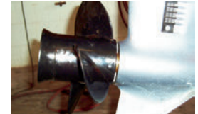
Fig. 3 Failure to install gearcase adapter ring leaves gap that causes excessive ventilation, poor performance.
